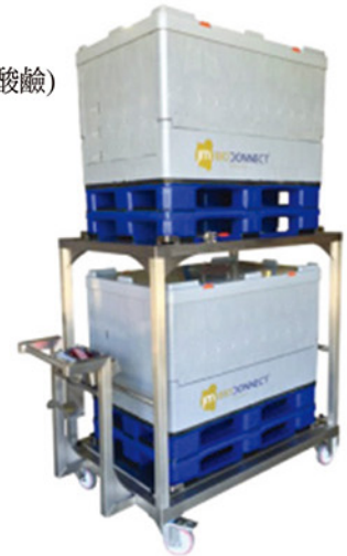
● Two 500 L containers stacked on weighing trolley
