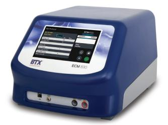
The ECM<sup>™</sup> 830 is designed for a wide variety of in vitro and in vivo electroporation applications. BTX square wave technology provides the advantages of high transfection efficiency and high cell viability for numerous cell and tissue types. Applications of the versatile ECM 830 for gene, drug and protein delivery include mammalian cells, in vivo and ex vivo tissues, zebrafish tissue and embryos, plant protoplast, and basic bacteria and yeast transformations.
